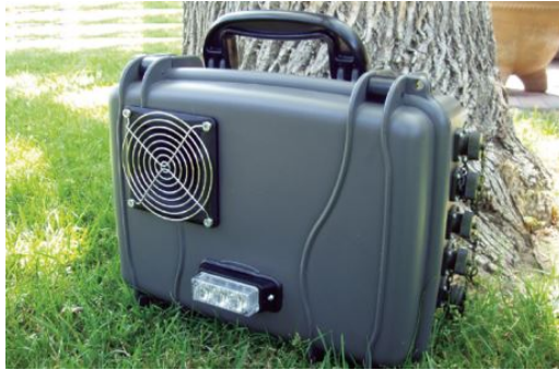
Picture 9: The ScareCall, a fully programmable light and sound device that can be suspended on a fence or tree in a pasture to prevent the advance and intrusion of wary carnivores. The device can use randomly activating lights and repellent sound effects.
